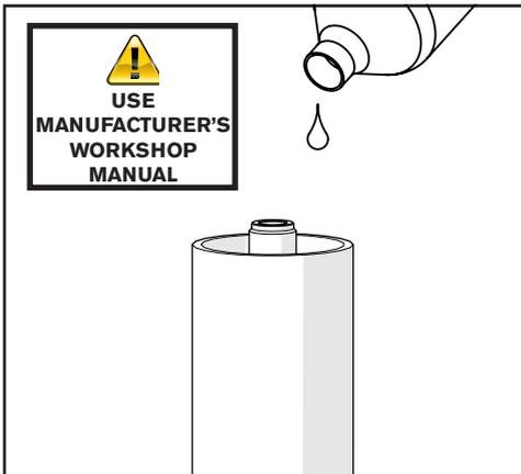
Pour in fork oil to level recommended by manufacturer. You may need to pump the fork up and down whilst doing this to allow the oil to settle.
