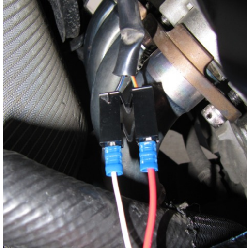
Figure 5 - Horn connector with harness installed
