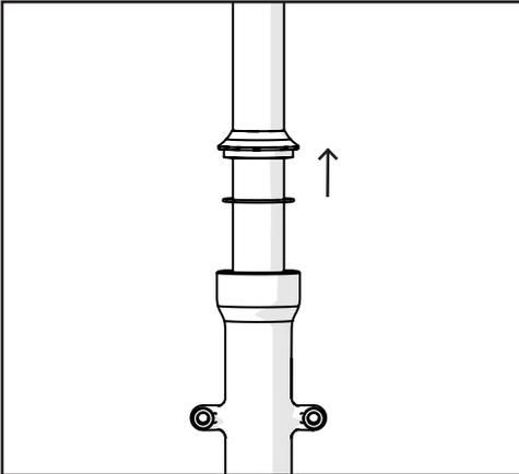
Remove Dust Seal and C-Clip.
