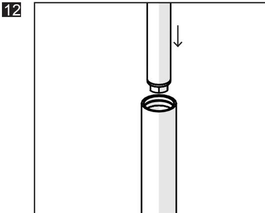
Install the cartridge into the fork leg.
