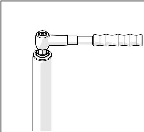
Screw the top cap onto the outer tube and torque to 10Nm using tool no. 113-010-115.
