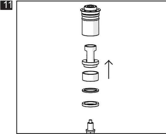
Remove the Top cap from the piston rod along with the nylon pusher, two preload spacers and the spring seat washer. To remove top cap use 14mm spanner to hold the rod and a 14mm socket on the centre of the top cap.
