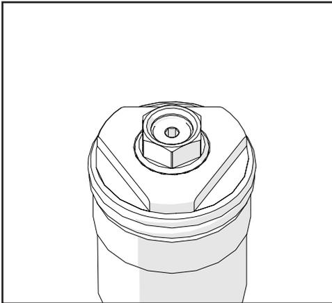
Set your compression and rebound adjusters using a 3mm allen key in the centre of the top cap. Adjust your preload using a 14mm spanner on the centre of the top cap. Make reference to the setting data in this manual.
