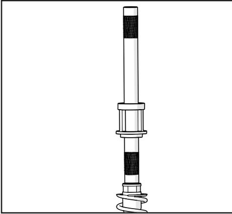
Pull the piston rod up using tool no.113-030-005 and install the nylon preload pusher.
