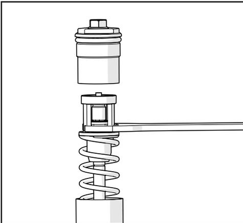
Holding the piston rod up with tool no. 113-030-005 place tool no. 113-010-020 onto the rod joiner and hold in place. Remove the pull up rod and install top cap.
