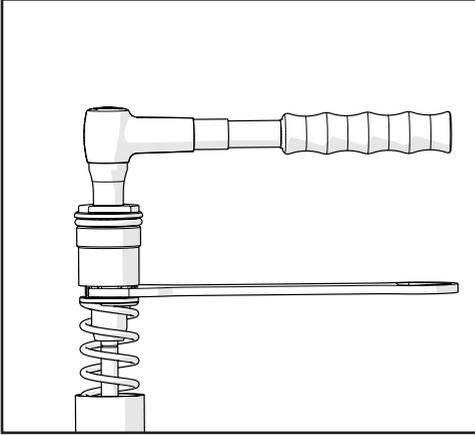
Torque the top cap onto the rod using a 14mm spanner and a 14mm socket, Torque to 12Nm.
