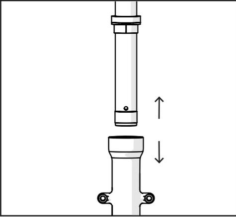
Remove the inner tube along with seals and bushes.
